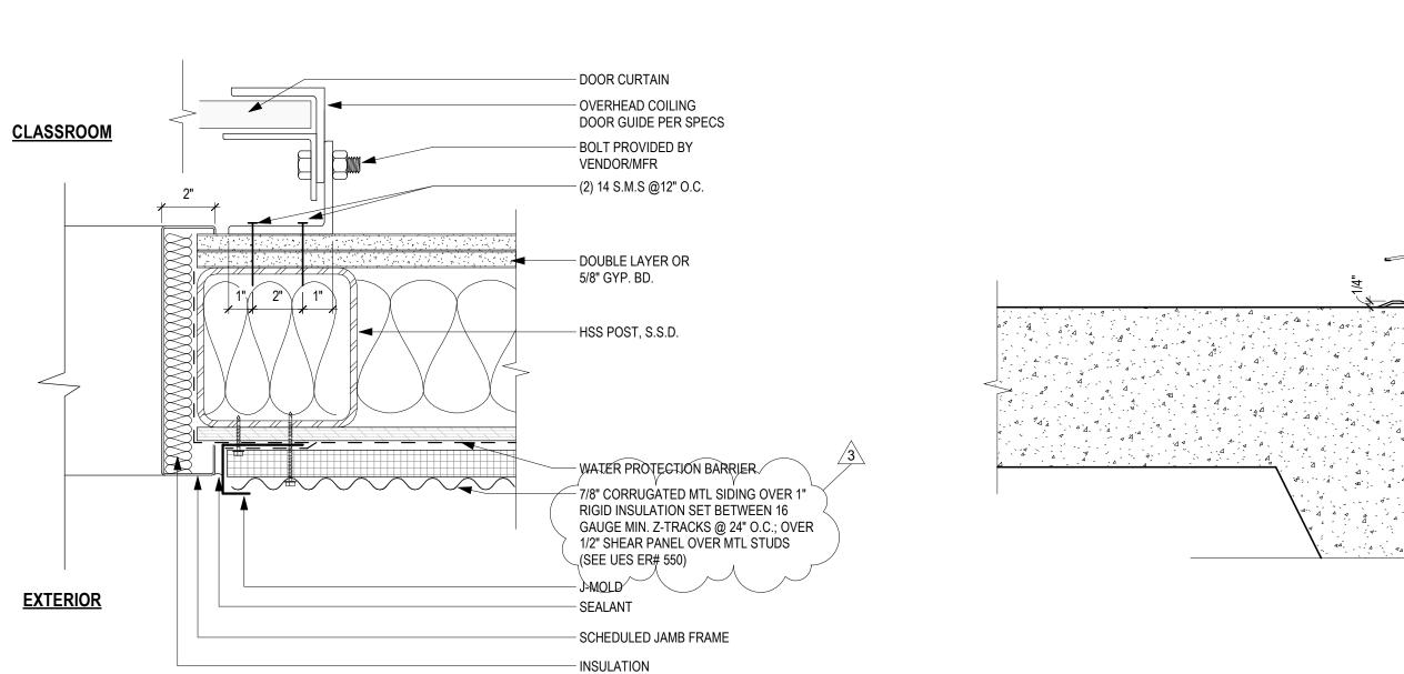
9 OVERHEAD COILING DOOR JAMB DETAIL
