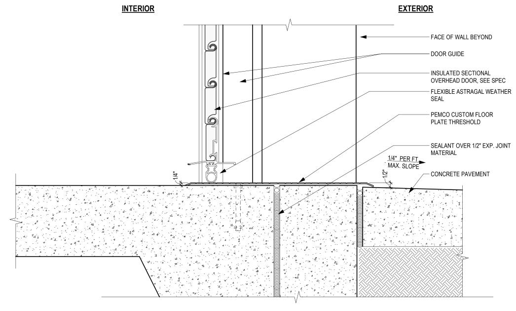
**OVERHEAD COILING DOOR SILL DETAIL**
