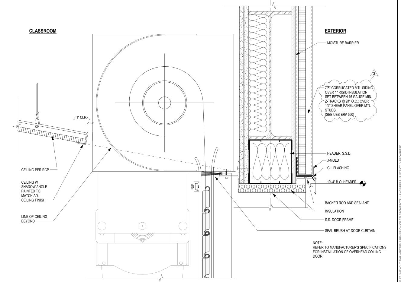
**OVERHEAD COILING DOOR HEAD DETAIL**
