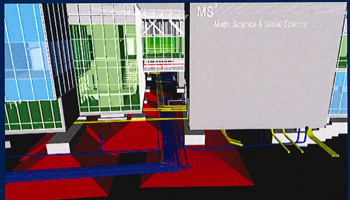
A model from the MS3 Building at Evergreen Valley College where there was a new utility trench that ran along the north side of the building. The utilities then ran through the breezeway which is where we needed to make sure they stayed above the plane of influence. We always model the foundation plane of influence to make sure any underground utilities are not impacted by the building's footings.
