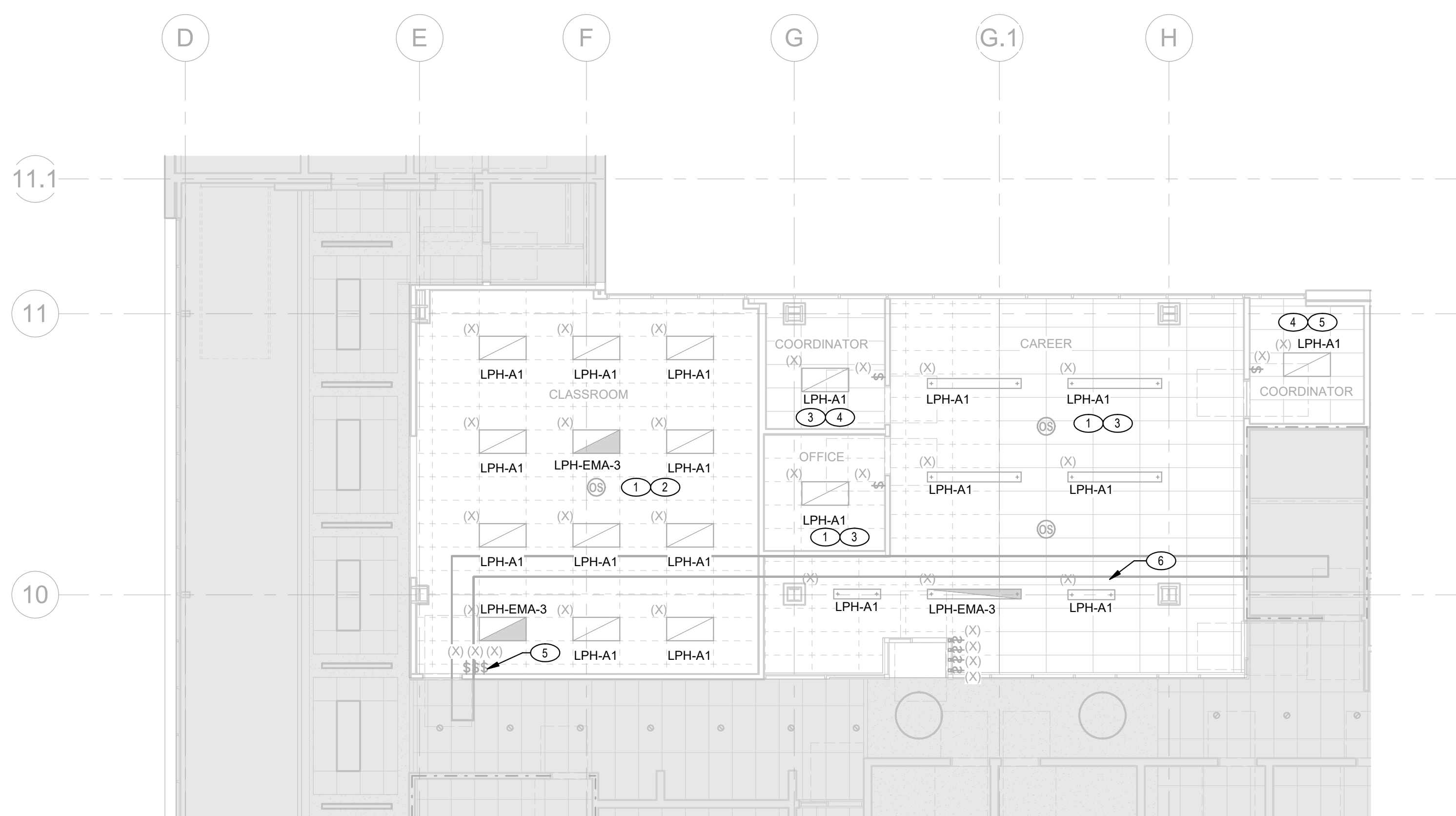
1 ELECTRICAL DEMO REFLECTED CEILING PLAN SCALE: 1/8" = 1'-0"
