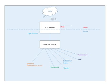
This architecture provides more control and analysis of traffic. It also provides for more robust failure recovery if one set of firewalls were to become compromised in any manner.
